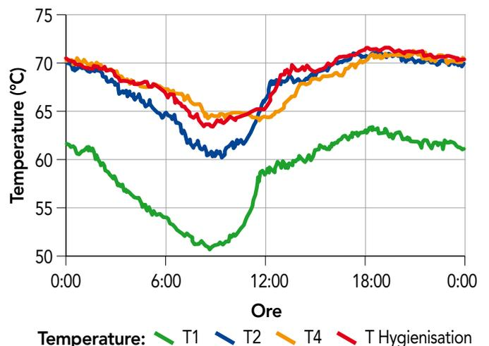
It is easier to maintain the process temperature during the spring, but the increased temperature range produces oscillations in the process controls.
