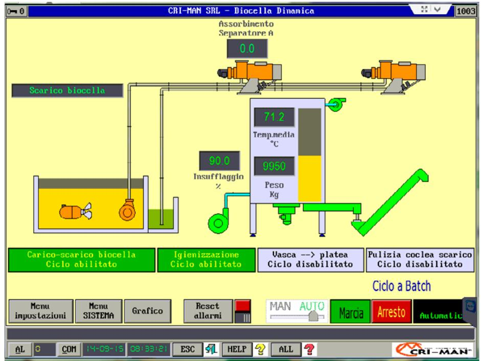
The main page of the management software displays all the components of the HBC separation system with continuous updating of the process data (temperature, weight, air input)
