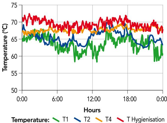
Low winter temperatures make it more difficult to achieve the sanitization temperature (red line), but by adjusting the unloading rate and air input it is still possible to achieve the required conditions.
